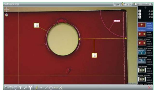
Holes dimensional data on an aerospace component.
